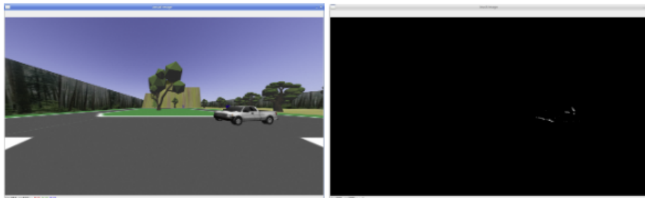
Fig 10 - left picture is the truck on robot camera image and right picture is the HSV mask
