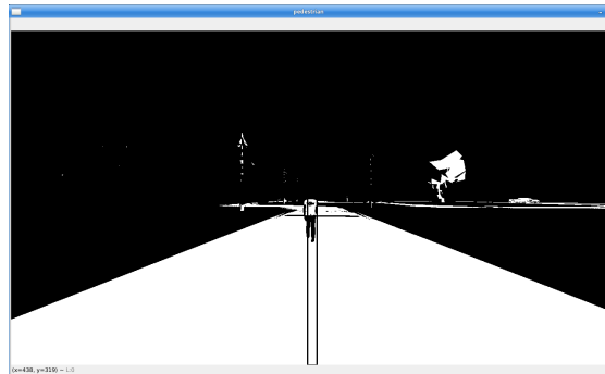
Fig 9 - Pedestrian being detected, the black vertical rectangle is the region that the robot is looking for variations
